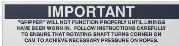
Figure 17 – IMPORTANT – Lining Wear-In
