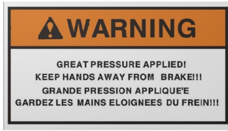
Figure 27 – Movable Shoe Warning Label
